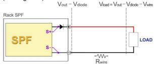
**Figure6** – In an SPF system, the voltage sensing is always positioned upstream of the decoupling diodes, so it is not possible to compensate the voltage drop on the decoupling diodes or on the connecting cables.
