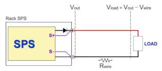
**Figura4** – In a standard SPS system, voltage sensing takes place on the output terminals of the rack. The voltage on the load is equal to  $V_{out} - V_{wire}$  (NOTE:  $V_{wire}$  = voltage drop on the connecting cables).
