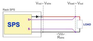
$\mbox{Figure5}$  – In an SPS system with  $\mbox{Sense Remote}$  option, the voltage sensing is brought directly to the load, to compensate the  $V_{\mbox{wire}}.$
