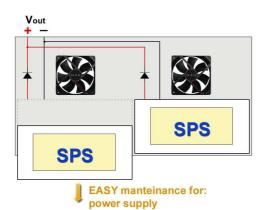
Figure2 – HOT SWAP of SPS modules, however the fans and the decoupling diodes are not easily replaceable.
